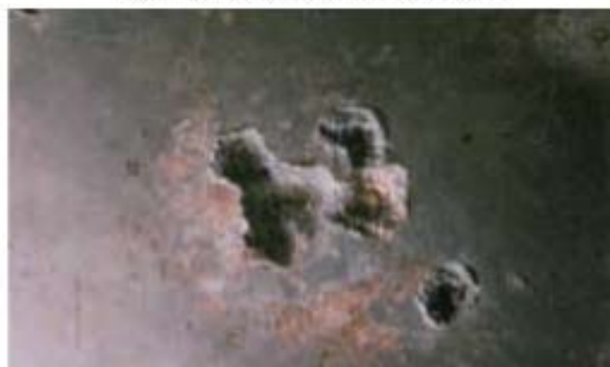
Fig. 2: Surface corrosion of a ship's tank
