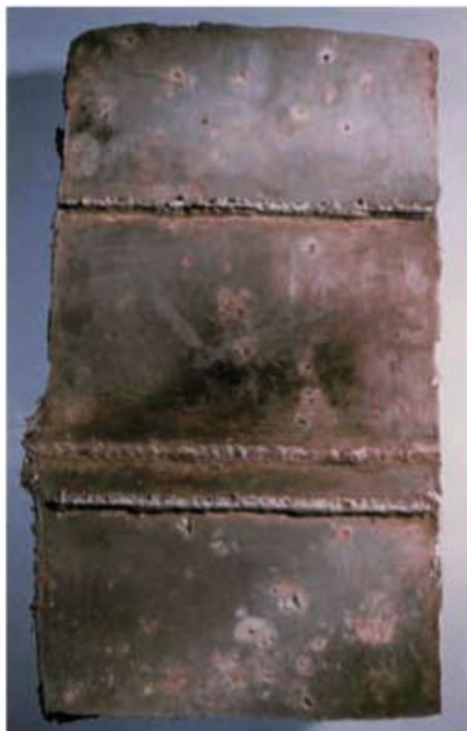
Fig. 2: Surface corrosion of a ship's tank
